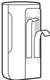
Peel the protective liners from the tape exposing the adhesive.
