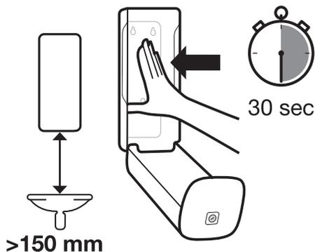
Mount the dispenser to the flat surface, press firmly and hold in place for at least 30 seconds.
