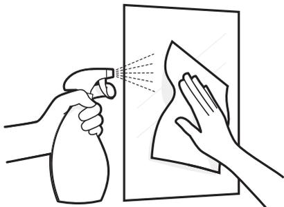
Ensure the mounting surface is flat, clean and dry.
